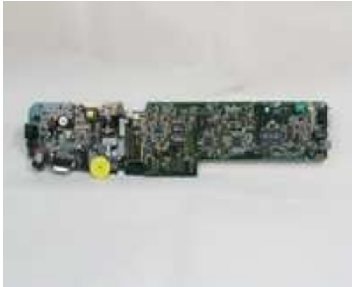
Main Board PWA 101-200. PCB 300-301. Assembly 399-708
