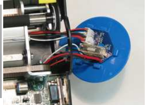
Fuse board and battery connection
