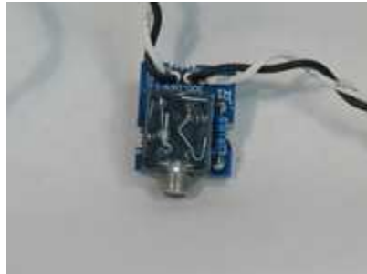
Earphone PCB assembly 399- 703
