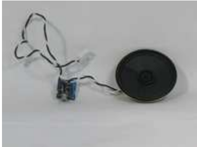
Earphone /Speaker PWA 101-009 (fits behind Left hand end cap speaker grille).
