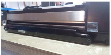
6. Using the two screws provided with the module attach the module to the body of the unit.
