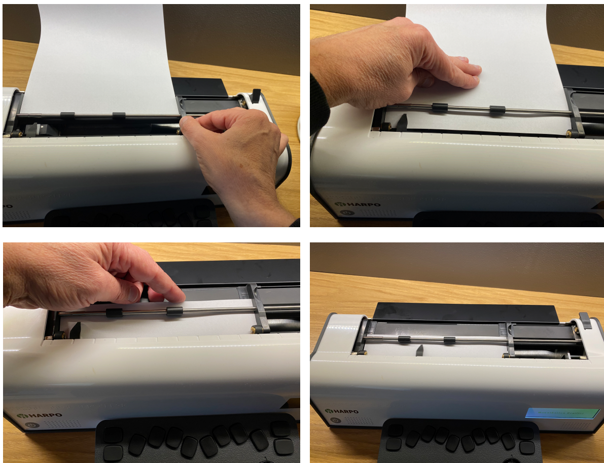
Fig. 5: The four steps for loading paper into the MB Tutor.
