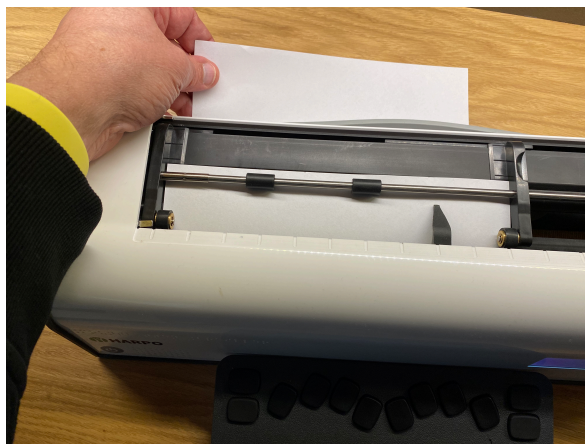
Fig. 6: Loading paper from the back of the MB Tutor
