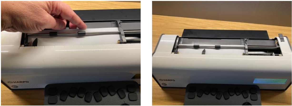
Fig. 5: The four steps for loading paper into the MB Tutor.
