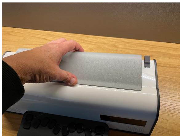
Fig. 1 Removing the top cover of the Mountbatten Braille Tutor
