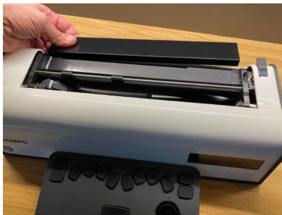
Fig. 3 Installing the Reading Table
